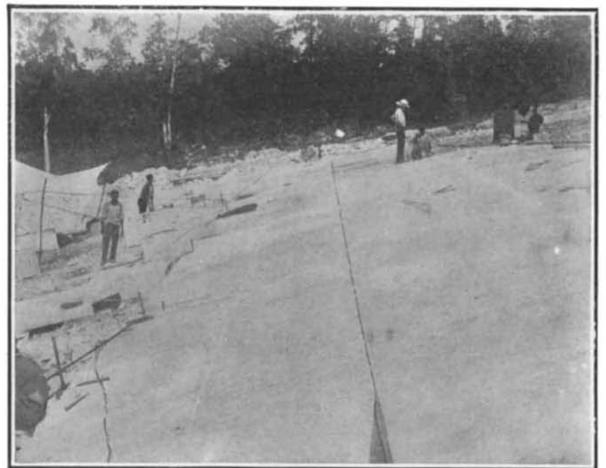
A "lit" being split and drilled into required widths and lengths. THE "LIFTING PROCESS" IN THE QUARRYING OF GRANITE.
