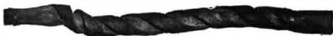
Vanadium steel, 3/4 twists in 2 1/4 inches. Elastic limit of torsion 7,540 inch pounds. Ultimate torsion 30,700 inch pounds.
