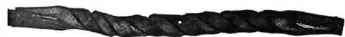
Carbon, high Manganese steel, 3/4 twists in 2 1/4 inches. Elastic limit of torsion 3,700 inch pounds. Ultimate torsion 17,250 inch pounds.
