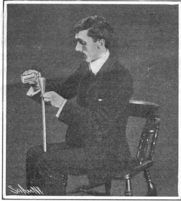
Filling the Mercury Tube.
