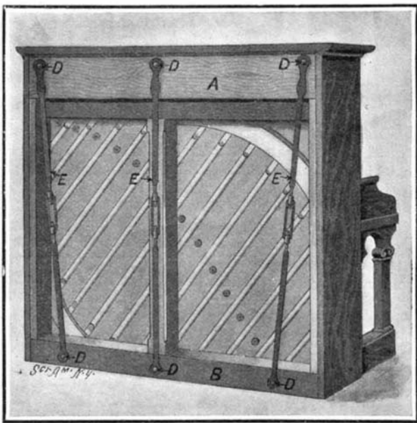
ADJUSTABLE TENSION RODS FOR PIANOS.
