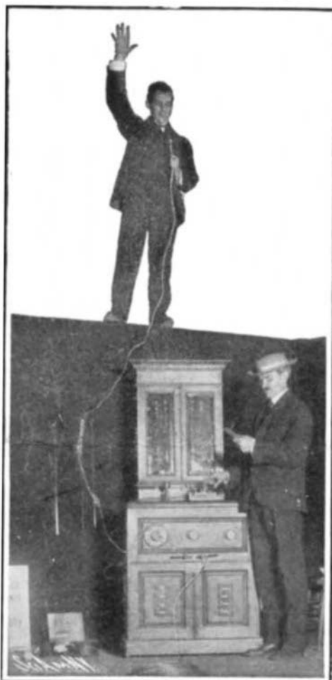
USING THE HUMAN BODY FOR SENDING A WIRELESS MESSAGE BY THE DE FOREST SYSTEM WITH THE ASSISTANCE OF DR. OVINGTON'S MACHINE. IN THIS EXPERIMENT 200,000 VOLTS OF HIGH FREQUENCY CURRENT ARE PASSED THROUGH THE HUMAN BODY, WHICH SERVES AS A MAST.
