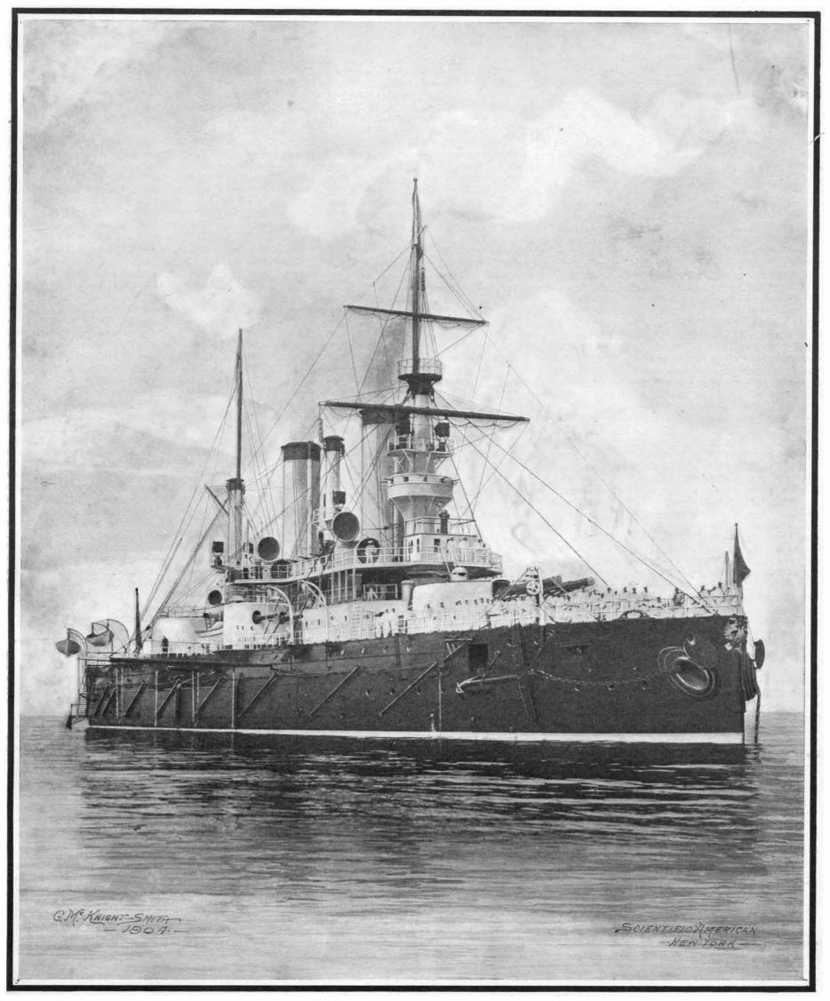
Copyright, 1904, by Munn & Co. Displacement, 11,000 tons. Speed, 17 knots. Armament: Four 12-in., twelve 6-in., 37 smaller guns. Armor: Partial belt, 15-in.; main turrets, 10-in.; smaller turrets, 6-in.; deck, 314-in. Torpedo Tubes, 6. BATTLESHIP "PETROPAVLOVSK," BLOWN UP AT PORT ARTHUR, WITH THE LOSS OF ADMIRAL MAKAROFF AND 750 OFFICERS AND MEN.-[See page 327.]
