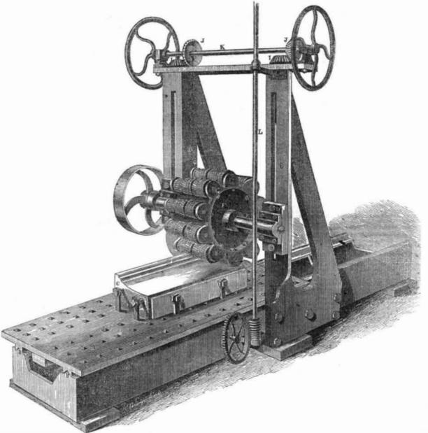
grooved or burred faces, made of cast iron and with bevel pinions, J J, meshing into others, I chilled, are strung, as it were, on a series of I, on vertical spindles, which have screws spindles, around a drum; the drum is revolved, upon them working into nuts, (not shown,) and are a composite of iron and steel. and the stone to be dressed is fed forward to it, on the inside of the boxes, D', for raising when the burring tools dress stone, by abrasion.
