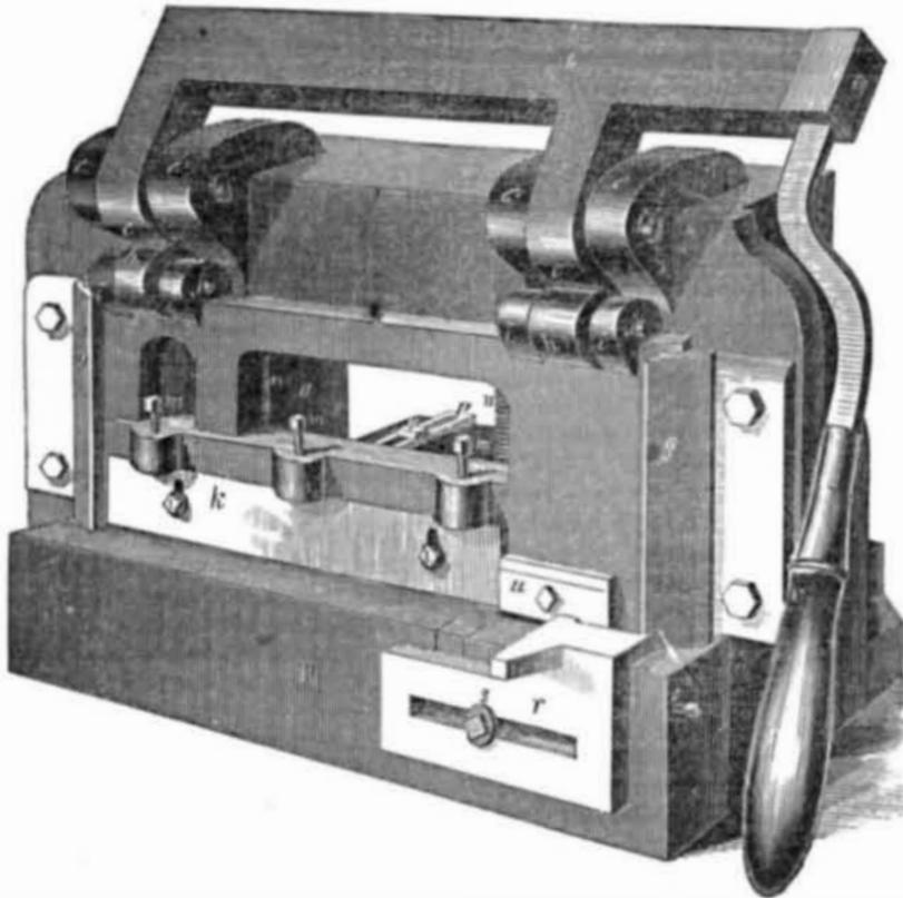
The annexed engraving is a perspective view of a machine for cutting out the corners and securing the edges of paper for boxes, for which a patent was granted Dec. 4th, 1850, to Andrew Dennison, of Brunswick, Me.
