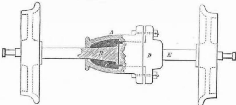
The annexed engraving is a front view partly in section, of a car axle, invented by S. L. Denney, of Christiana, Lancaster Co., Pa. The object of this axle is to give to each wheel an independent motion to allow the wheels of cars to accommodate themselves to the curvatures of tracks. One of these axles is on exhibition in the Crystal Palace.
