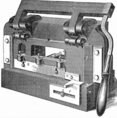
of a machine for cutting out the corners and se- In front of the die is another gauge, r, at right curing the edges of paper for boxes, for which angles with p: it is secured to the bed plate a patent was granted Dec. 4th, 1850, to Andrew Dennison, of Brunswick, Me.
