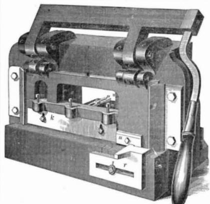
The annexed engraving is a perspective view | forth according to the size of box to be .cut.of a machine for cutting out the corners and se- In front of the die is another gauge,  $r_1$  at right curing the edges of paper for boxes, for which angles with p: it is secured to the bed plate a patent was granted Dec. 4th, 1850, to Andrew Dennison, of Brunswick, Me.
