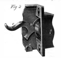
lower sash (when it is down), which is cut just deep enough to let the eccentric roller, A, turn down, until the lever hooks, with its catch, D, into the wedge-shaped space, E, behind a small projection on the face plate. The sash is now fitted, and the window complete.
