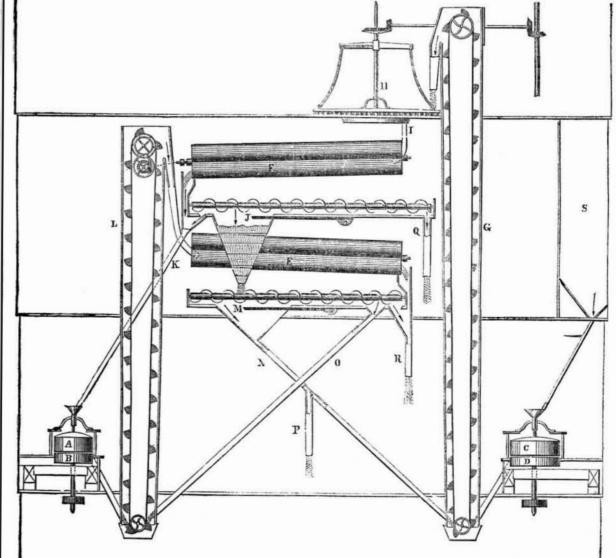
tion of a mill, which illustrates the process of ary mill, A B, to hold a few bushels of offal, so flouring, for which a patent was granted to Da. that any irregularity of the supply from the bolts vid P. Bonnell, of Indianapolis, Ind., on the may be overcome and the stone not be permit-14th of August, 1849, and re-issued on the 5th ted to run dry. The bolt cloth for this plan of last July
