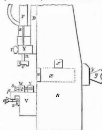
so adjusted that the drill or chisel will pass between them when it goes through the piece. The stop, Z, is set to prevent the piece from being lifted by the tool, when raised to draw it out. The score, Z', in the stop, Z, allows the ends of the chips in the mortise, which project above the surface of the piece under operation to pass freely. When the piece to be mortised is reversed, the chips come between the bars,
