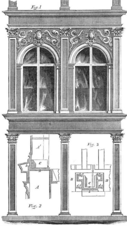
The annexed engraving illustrates an im- are secured thereto by bolts and nuts, c c, for iron building constructed according to this imthe second story, as it would appear when fin- or contraction of the summers may be allowed. the improvement claimed; and fig. 3 a plan A', the chairs should severally be adjusted to view of the same. Similar letters of reference
