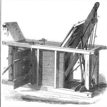
The rope, P, is connected at one end to the scantling of the frame, and down over another pulley. This cord is for drawing back the follower and elevating the levers, when the cotton or hay is pressed and secured in bale. This It is a very simple press, indeed, and as we Albany, N. Y.
