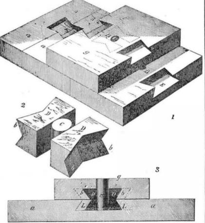
tion of an improvement for locking stones for the foundations of such structures as lighthouses, bridges, &c., for which a patent was granted to John P. Avery, on the 25th of last April (1854.)
