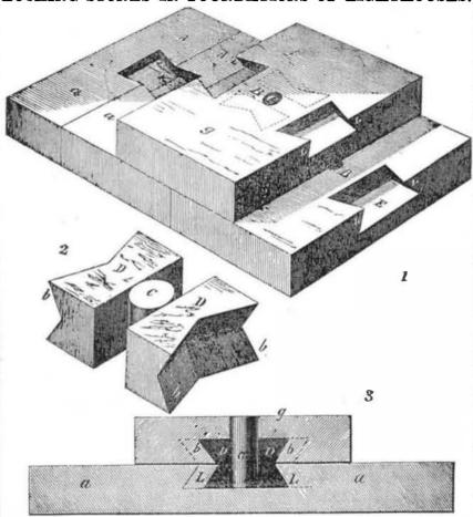
We herewith present an illustrated descrip- | with the stone which breaks joint with them tion of an improvement for locking stones for the foundations of such structures as lighthouses, bridges, &c., for which a patent was granted to John P. Avery, on the 25th of last April (1854.)
