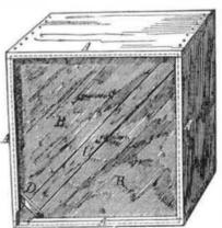
The annexed figure is a view of an improvement in the construction and fastening of lids of packing boxss, &c., and the same plan may also be applied to barrels. A is a box, represented with a croze around its interior sides near the top, for the reception of the two angular parts, BB, which forms the lid. A bar, sending milk mixed with water.
