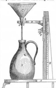
A represents a platform or base on which are placed two vertical guides, B, between it firm in its socket, and serve to arrange the which a frame, C, works, one guide only is
