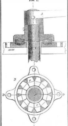
The nature of the improvement consists in the employment of a series of rollers made in the form of double frustums of cones united at their bases, and adapted to run in grooves of nearly corresponding form made in the surfaces, between which they are interposed.
