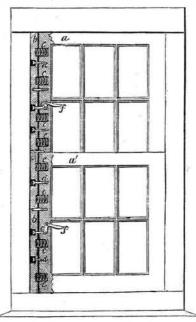
a a are the upper and lower frames of a window. Into one side of the sash is made a groove, and into this is let the expanding sash, b, which is a strip of wood. Small recesses or holes are cut in the sash of the window, and into these are placed coiled springs, c c. The expanding sash is secured by screws, d d, to the window sash. This expanding sash, owing to the tension of the springs, c c, presses against the side of the window casing, and holds the window in any position in which it may be
