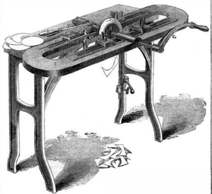
observed that the cutting pollers cut it off, roller, R is moved around against it, and turns forming it into a disc. The waste pieces are shown below the table.
