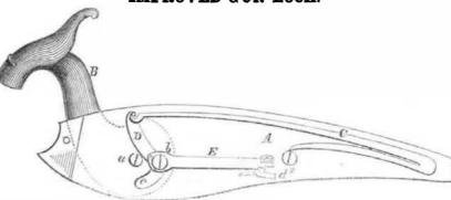
August. This figure is a view of the inner side plate, fully protected from moisture. of the lock-plate, showing most of the parts of
