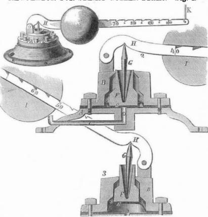
The annexed engravings are views of an improvement in Regulating the Dampers of Steam ing the damper in the chimney (or if a blower Boilers by the pressure of the steam, for which is used, the damper for shutting off the blast,) a patent was granted to Patrick Clark, of Rahway, N. J., on the 3rd of last January.
