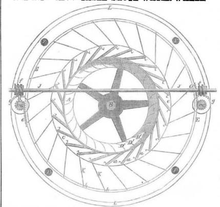
The annexed engraving is a bird's-eye view, | ter and speed of the Howd or United States with the upper rim removed, of an improvement in adjustable shutes for water wheels, for which a patent was granted to Elijah Roberts, of Rochester, N. H., on the 4th of last month (April, 1854.)
