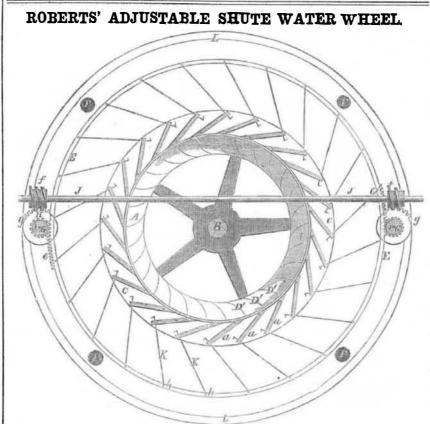
with the upper rim removed, of an improvement in adjustable shutes for water wheels, for which a patent was granted to Elijah Roberts, of Rochester, N. H., on the 4th of last month (April, 1854.)
