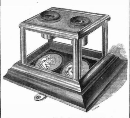
Mascher's new Stereoscope, designed for Da- cher's Stereoscopic Daguerreotype Case, patentguerrean artists. It is constructed of plate ed March 8th, 1853, and illustrated in No. 37 of glass mounted with German silver. Two tubes our last Volume. These cases, we understand, are seen, which contain the lenses, and may be are being rapidly introduced, and we certainly screwed in or out to accommodate the vision of think that no one, having seen them, will have different persons.
