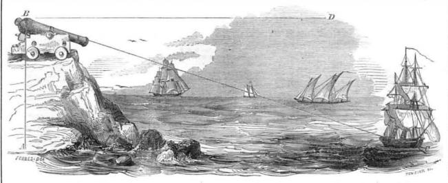
to A B, so is radius to B C the inaccessible distance. Thus we obtain a common formula, namely, that the hight of the piece above the of depression will in all cases give the distance of the inaccessible object from the gun.
