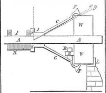
collar, O a double toggle, T, is applied for moving each pair of wheels backwards or forwards simultaneously upon the axle. In practice, however, it may be found that converging grooved rails upon a track of sufficient length will answer the purpose as well. That part of each case, S, near the central collar, is made to project, in order that a suitable key may be applied to clamp each pair of cars together to the narrow, and key them apart to the widest
