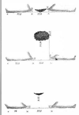
The shot passed through the  $4\frac{1}{2}$ -inch plate and rubber, and penetrated the timber the same as previous shots fired at other targets made in the usual way without rubber, the only exception being that the target was thrown on its face at both fires.
