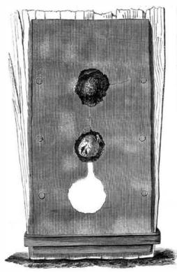
DIMENSIONS OF PLATE.—8 feet 3 inches long; 4 feet 2 inches wide; 4½ inches thick. Gun, XI. inches, Charges, cannon powder, 1862. Projectiles, Cloverdale cast-iron solid shot. Primers friction tubes.
