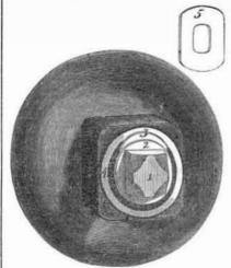
After the bolt and nut have been screwed to their places, the washer, 3, is shoved up as represented in the cut, and the bolt, 1 screwed tight. This washer thus projecting prevents the nut from unscrewing and working off the axle. This plan will be readily understood without further description, is simple and cheap and we should think if properly carried out it might be efficient.
