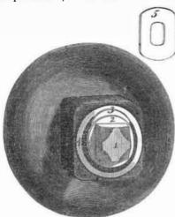
After the bolt and nut have been screwed to their places, the washer, 3, is shoved up as represented in the cut, and the bolt, 1 screwed tight. This washer thus projecting prevents the nut from unscrewing and working off the axle. This plan will be readily understood without further description, is simple and cheap and we should think if properly carried out it might be efficient.
