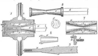
washers will be required, and the wear at the opening in the end of the hub, so as to give a ends of the hubs will hardly be perceptible, as neat exterior finish, and prevent the entrance the cones. An equal and constant supply of the hub and axle when necessary. oil will be obtained, thus insuring them against grinding and heating.
