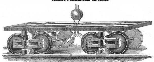
The engraving annexed is an illustration of a | and middle cross ties; D D are the axle ties, as a support when a wheel or axle is broken; as a Track-Keeper when obstructions are on the track or in case of collisions: as a protector of wheels and axles, by relieving them of their weight in all emergencies, and as a preventive of collisions by serving as a more effectual brake.
