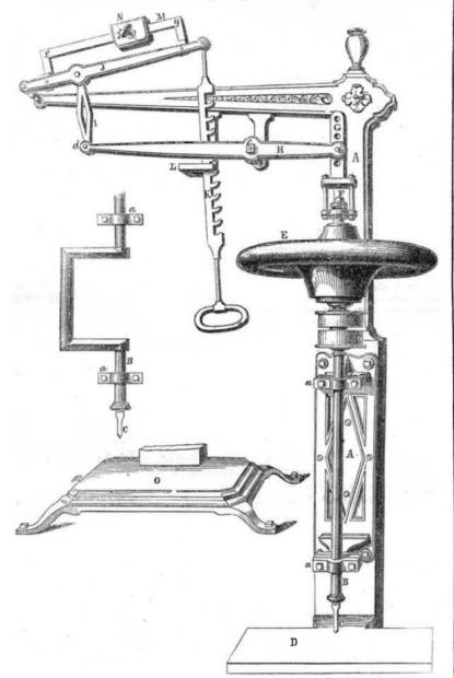
The engraving presented on this page is an secured firmly to the rod, M, at any desired illustration of a drill, for which a patent was granted to Warren Lyon, of this city, Septemthe implement consists in having a weight atpose of giving the requisite pressure, and in having a system of levers and a counterpoise connected to the upper part of the arbor, for the purpose of elevating it and graduating the pressure communicated to the drill by the weight upon the arbor.
