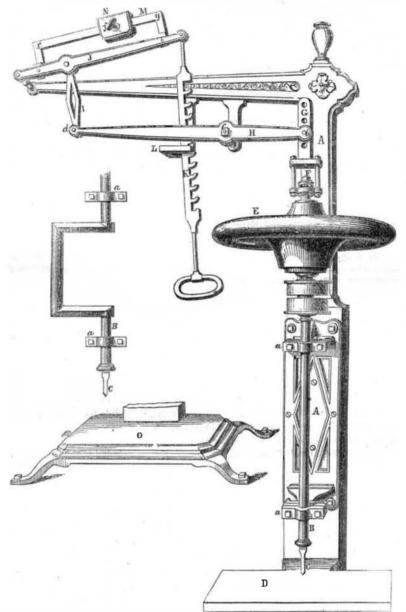
illustration of a drill, for which a patent was granted to Warren Lyon, of this city, Septemthe implement consists in having a weight atpose of giving the requisite pressure, and in having a system of levers and a counterpoise connected to the upper part of the arbor, for the purpose of elevating it and graduating the pressure communicated to the drill by the weight upon the arbor.
