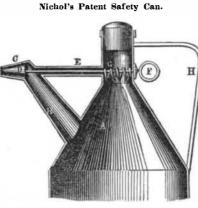
The annexed engraving is a perspective view of the ordinary decanting vessel, with a sectional view of the tube, showing Nichol's im-
