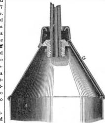
also frequently takes place at the side tube used for filling. The tin tube being soldered to the cap, when any sediment from the oil gets into the tube and stops its running, it has to be forced back into the can by means of a wire, and of course is liable to trouble again. The tin tubed cans and all others however constructed, except this, are frequently covered with oil, dripping down on the outside, rendering them dirty, and wasting much oil.
