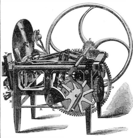
cess of a tobacco-pressing machine. If the to-, tance between the back and front ends of the the plugs under pressure while confined for pressing power. about half an hour, during which time the plugs lose their elasticity, and always retain their form after they are discharged. This machine presses about 20 plugs per minute, and the receiving as it is somewhat long. When full, as one pressed plug is thrust in by the lever Y, one is
