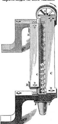
The annexed engraving is a plan view of an of the pressing vell-the plate wheel, W, is kept improved hopper for feeding blanks into screw
