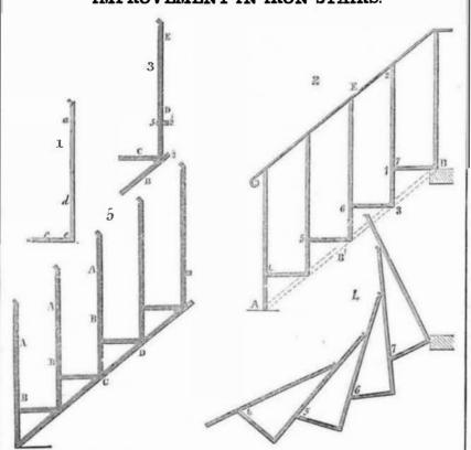
The annexed figures are views of an im-tiron is formed the baluster, a d, (figure 1) fits over a projecting arm, m, in the hinged of iron bars, to form a stair. Out of a bar of is a tennon on the other end to be inserted
