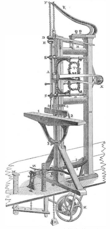
The above is a perspective view of Otis' on the [chisel rod because the centre of the Mortising and Boring Machine in combina- pin in the sliding fulcrum, L, is cut away, tion. A represents the mortising or chisel thus causing the centres of motion to be dishaft, B, the boring or auger shaft.
