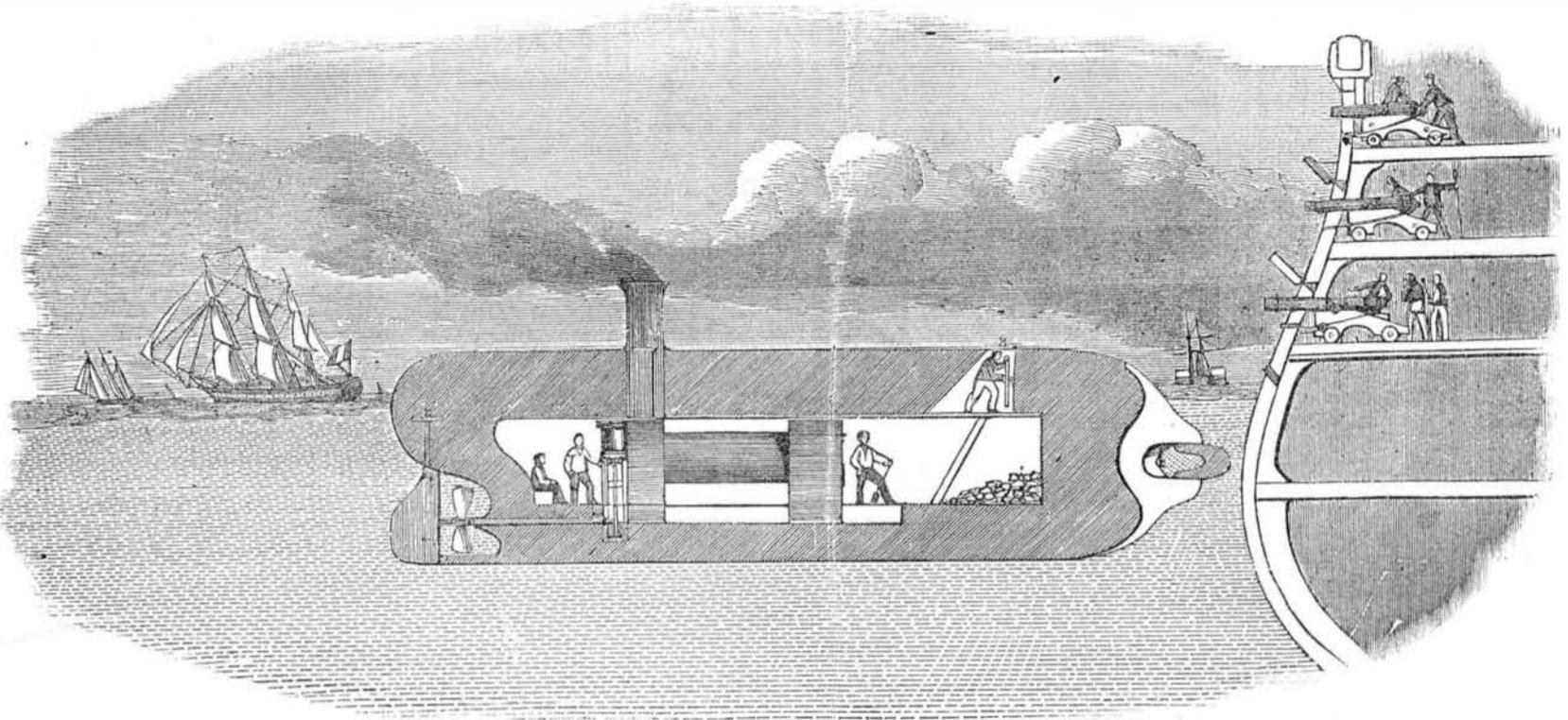
The annexed engravings are views of a floating, partly submerged Propeller, Torpedo Vessel, proposed by James Nasmyth, of Patricroft, England, for destroying large ships of an invading fleet.
