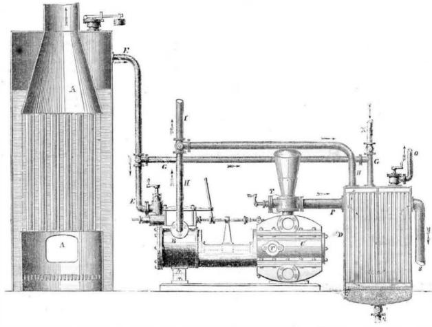
The annexed engraving is an elevation partly in section, of a boiler, Worthington & Baker's steam engine pump, and a condenser, combined and arranged in such a compact manner by Charles W. Copeland, engineer, of this city, as must commend the same to the general attention of all concerned .-For ship's it is a most commendable apparatus, and should be employed in every one that sails on the ocean; no whaling ship, at least, should be without such apparatuses.
