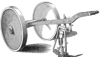
This engraving is a perspective view of a | throwing it out at the side of the ditch. The machine for digging ditches, invented by Jo- | plate, P, is but to incline the sod to the one nathan W. Morrill, of Hampton Falls, N. H., side. who has taken measures to secure a patent for the same.
