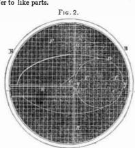
A represents the upper part of the smoke pipe; it passes into the main funnel, B. C C are exhaust tubes, which pass upwards in the smoke-pipe, and terminate a short distance below its top. D is a shield placed over the smoke pipe a short distance above it; this shield is attached to a vertical partition, a, in the centre of the funnel. E is a chamber, the top of which extends from the partition, a, to the side of the funnel, B. This chamber narrows gradually to the tube, b, which tube com-
