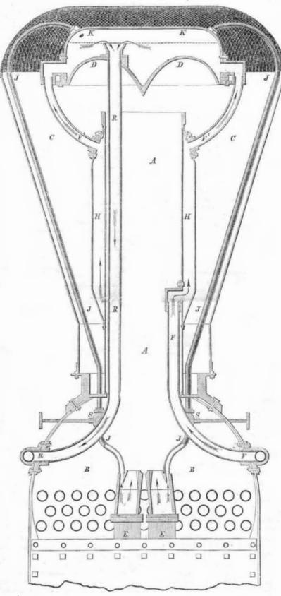
The above engraving represents a transverse | iron attached, also water tight, by a flange to ction of a locomotive chimney and smoke box and its exhaust steam |cone, and with it forming a water vessel of or blast pipes, with the Apparatus for Heating Feed Water attached thereto, invented by Israel P. Magoon, of St. Johnsbury, Caledonia H; F is a pipe (two inches in diameter) lead-
