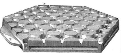
To supersede the ordinary Russ paving for mortice or groove, C, let into it, into which iron blocks has been invented by L. Colwell, of New York City, who has taken measures to secure a patent. The above engraving is a perspective view of one of the blocks forming a section of the paving and displays the structure and arrangement of this new method Each of these blocks is six-sided, being in shape a regular hexagon, so that they are easily fitted one to another.
