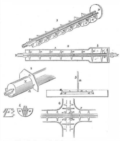
The annexed engravings are views of a | bar. This being accomplished, the upper part valuable improvement in the moulding of cast- or surtace of the core-bar is covered with iron tubes, invented by George Peacock, of green sand and piled up till it reaches a neces-West Troy, Albany Co., N. Y., who has taken measures to secure a patent for it.
