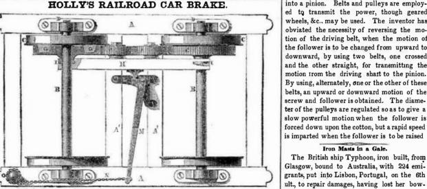
The figure shows a truck-frame, A A A' A'; on the cross-braces is secured a fulcrum plate, L, for the fulcrum pin, K, of the lever, M, which lever is operated by the brakesman with a vertical shaft, O, which winds up the chain, N, and pushes in a swinging clutch frame, H, by the bottom of the lever, at K, acting on the projection, J, which is at the bottom of the frame, H.
