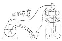
A is a tubulated retort filled with soluble glass; and B is a dish of mercury, in which positive platina wire, attached to the battery and dipping into the soluble glass in the retort; N is the negative wire connected with the battery, and forming a galvanic circuit with the positive wire by the mercury, and the wire in the retort.
