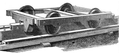
The annexed engravings are views of an | let us explain the new rails: C is a rail made invention for preventing locomotives and cars with a metal top and side flanges, B, (one not running off the track, also to improve the rails, in a very simple manner. The inventor is H. rail is keyed down on the sills in any Carpenter, of Rome, Oneida Co., N. Y., who proper manner, and projects like any other has taken measures to secure a patent for the rail. A is the truck; it is made in the usual
