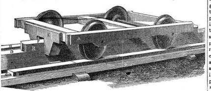
invention for preventing locomotives and cars with a metal top and side flanges, B, (one not running off the track, also to improve the rails, in a very simple manner. The inventor is H. rail is keyed down on the sills in any Carpenter, of Rome, Oneida Co., N. Y., who proper manner, and projects like any other has taken measures to secure a patent tor the rail. A is the truck; it is made in the usual same.
